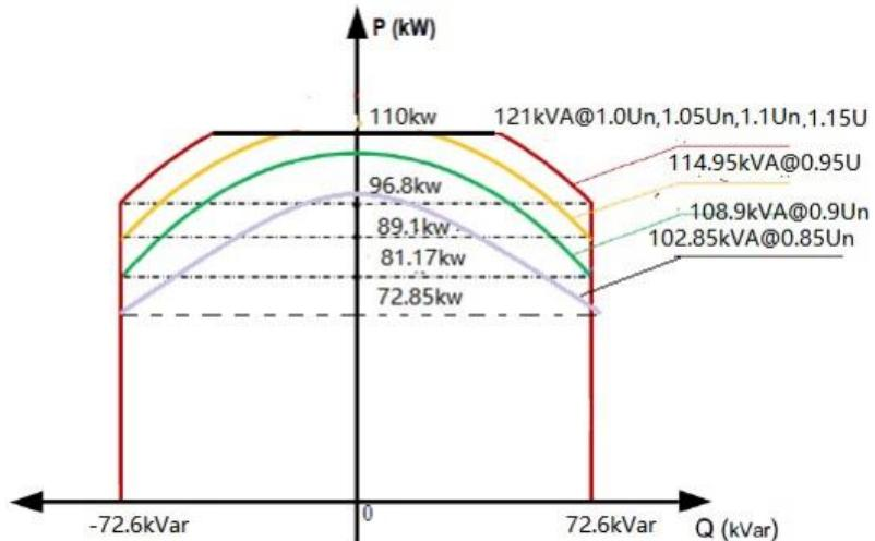
Figure 4 a. Voltage-dependent PQ diagram for R110
