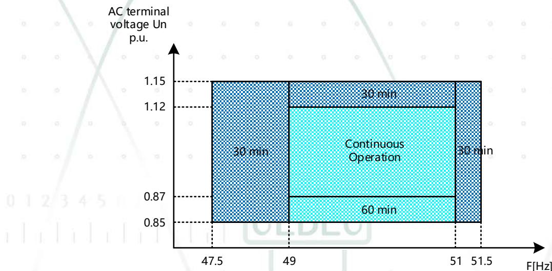
Figure 3 Quasi-stationary operation range for R SERIES PV
