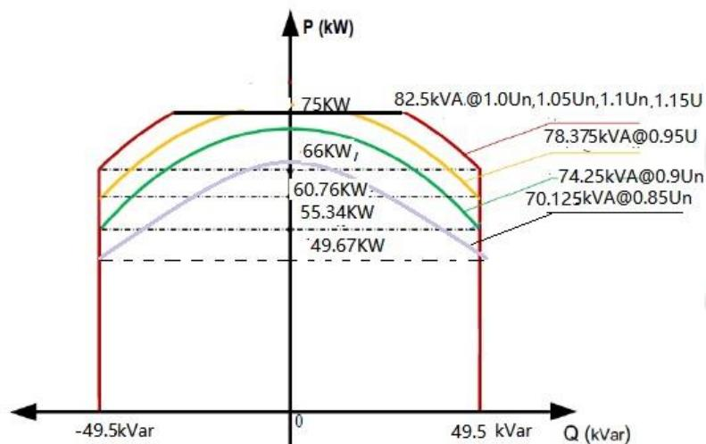
Figure 4. b. Voltage-dependent PQ diagram for R100
