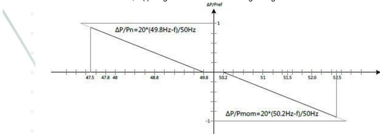
Figure 6 R SERIES PV P(f)-diagram
