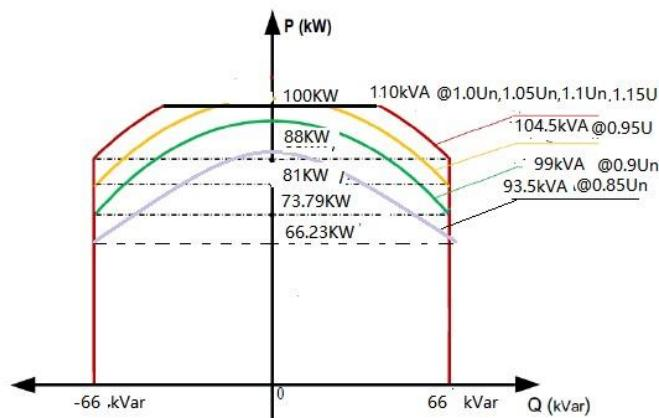
Figure 4.c Voltage-dependent PQ diagram for R75
