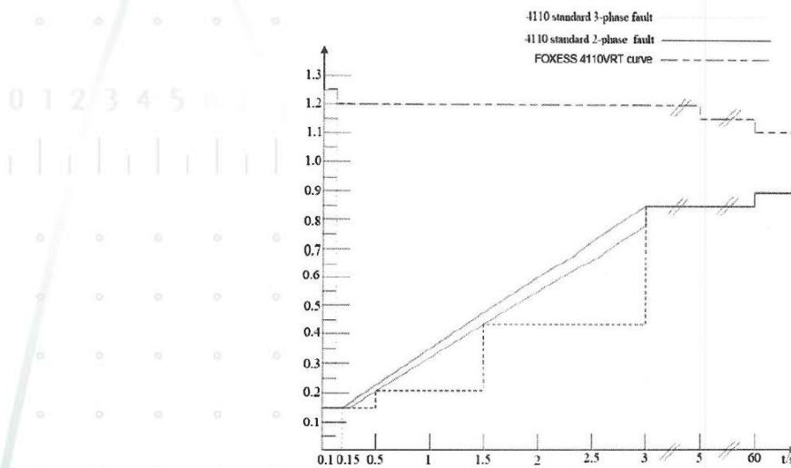
Figure 5 FRT limit curve for R Series
