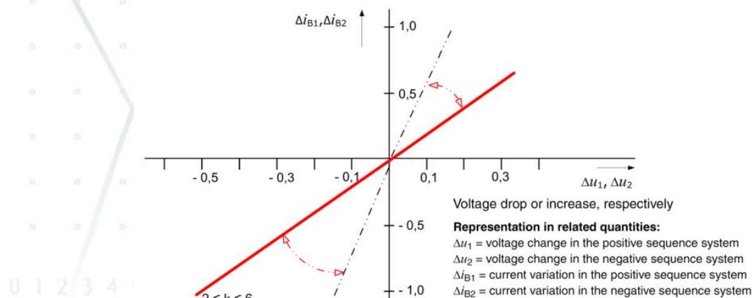
Figure 8 k factor of voltage support in the event of a network fault
